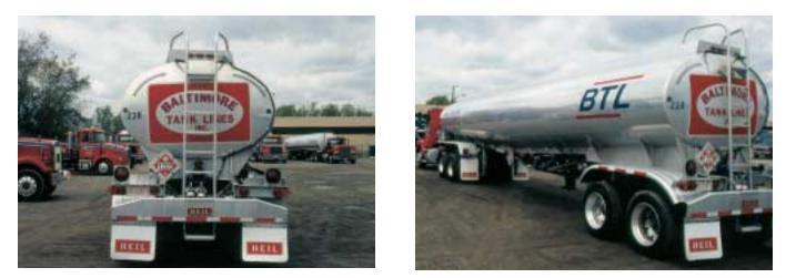
**Figure 25-44** The DOT-406/MC-306 is the most common truck on the highway today and is referred to as a gasoline tanker. It can and frequently does carry other types of flammable and combustible liquids. (*Photo courtesy of Maryland Department of the Environment*)
