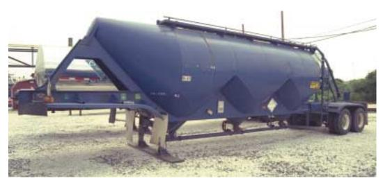
**Figure 25-58** Dry bulk tanks carry a variety of products. Some examples include fertilizers, explosives, and concrete.
