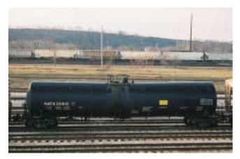
**Figure 25-63** The indication that this is a nonpressurized railcar is given by the fact that all of the valves are on the outside of the tank and not contained within any protective housing.
