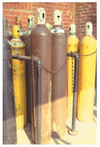
**Figure 25-37** Cylinders present additional risks to responders because not only can the contents be hazardous, but if the cylinder is involved in a fire it may explode.
