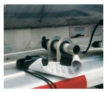
**Figure 25-43** In most cases the shipping papers will be with the driver in the cab of the truck, but they may be in a special tube located on the trailer.
