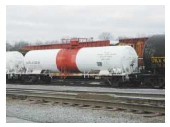
**Figure 25-64** This railcar is white with a red stripe, which is used to indicate hydrogen cyanide but on occasion is used to indicate dangerous materials. This car holds hydrogen fluoride anhydrous, which is a severe inhalation hazard and is corrosive. The term *anhydrous* indicates "no water" and means the hydrogen fluoride is pure.
