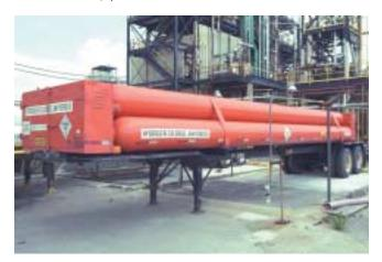
**Figure 25-57** The tubes on this trailer contain pressurized gases. The pressure can vary from 2,000 to 6,000 psi.
