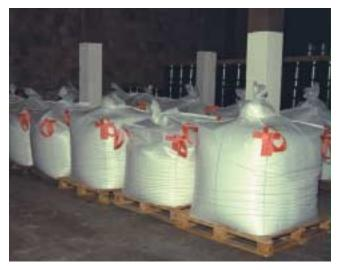
**Figure 25-36** It can be quite surprising to open the back of a tractor trailer and find these super sacks. They can hold solid materials, some of which can be toxic.
