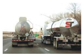
**Figure 25-48** On the right is an insulated MC-307/DOT-407, and on the left is an uninsulated MC-307/DOT-407. Both trucks hold comparable products, but the insulated one holds products that are heated or may require heating to offload.
