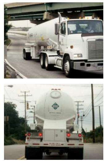
**Figure 25-53** MC-331 tanks carry liquefied compressed gases such as propane and ammonia. They are made of steel and are designed to carry a variety of products.
