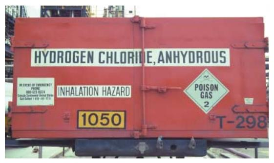
**Figure 25-24** The DOT adds the "Poison—Inhalation Hazard" label to those materials that present severe toxic hazards.
