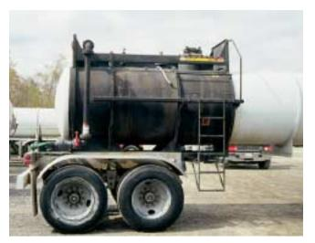
**Figure 25-52** The black coating around the manhole indicates that a corrosive is being carried. It is used to protect the tank from spillage. It is not required nor will it be found on all corrosive tanks.
