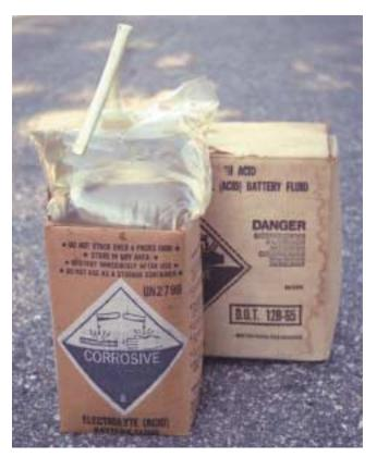
**Figure 25-33** Typically, chemicals that can cause harm are not packaged in cardboard. This sulfuric acid is one example of a material that can cause harm, but unfortunately is packaged in cardboard.
