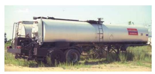
**Figure 25-59** These trucks carry molten products and can be heating the product while driving. This practice is illegal but is found on occasion. The fuels used to heat the product are either diesel/kerosene or propane.
