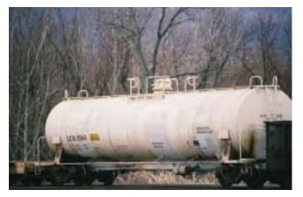
**Figure 25-66** This specialized railcar holds liquefied carbon dioxide, a cryogenic material.
