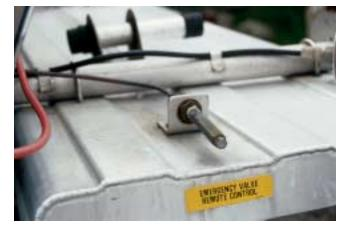
**Figure 25-47** On most trucks there is a minimum of one emergency shutoff, and with most there are two. The most common location is near the driver's door; the other is usually located near the valve area.
