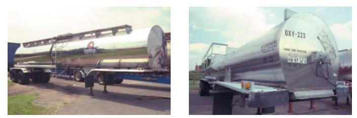
**Figure 25-49** This insulated version is identical to the uninsulated tank but has an aluminum cover and insulation. Note the differences in these two trucks. The one on the right has safety railings around the manhole. Although not an absolute rule, the truck on the right would carry more dangerous products and would have other added safety features. Most of these items are not required but were added by the trucking company.
