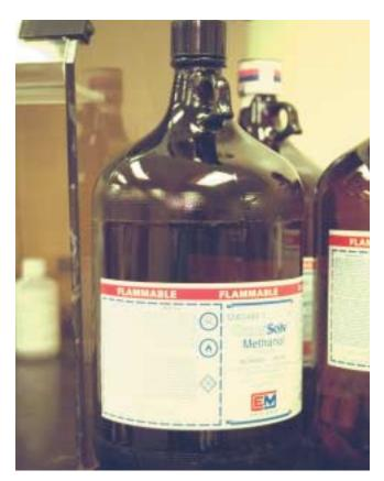
**Figure 25-35** This glass jar is coated with a plastic coating that will not allow the liquid to spill out if the glass is broken or dropped.
