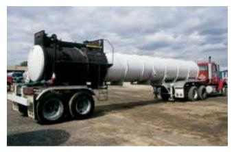
**Figure 25-51** The DOT-412/MC-312 is designed to carry corrosives and is similar in design to the uninsulated 307, although smaller. The inner tank may be lined with a variety of materials to prevent the corrosive from attacking the tank.
