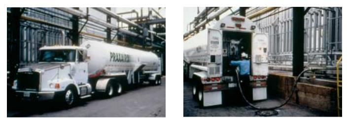
Figure 25-55 The MC-338 carries cynogenic liquefied gases. The tank resembles a rolling Thermos bottle.
