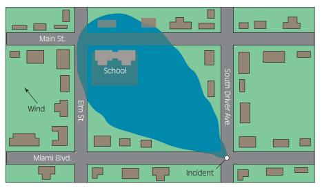
**Figure 25-38** The type of vapor cloud commonly referred to as a plume varies with the terrain and buildings in the vicinity. The plume here represents one of the most common types.
