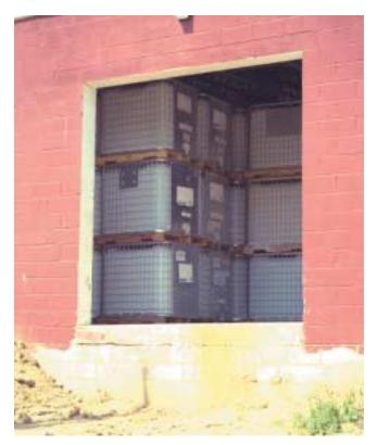
**Figure 25-39** The use of 55-gallon drums is decreasing and the use of these portable bulk tanks is increasing. Like the super sacks these can be hidden away in the back of a trailer.
