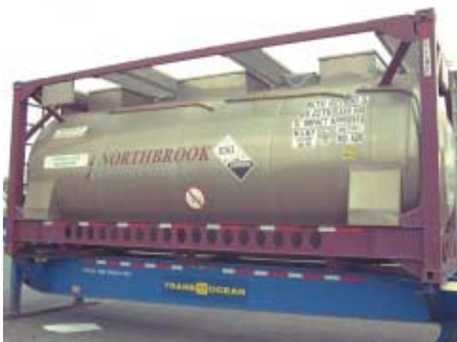
**Figure 25-60** This is an IMO-101 tank. Like the totes, these are bulk tanks capable of carrying a large quantity of product. These are normally placed on ships, then delivered locally by a truck, although trains can also be used.
