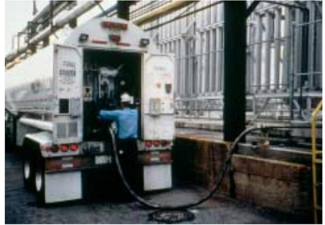
liquids, the material must be kept cool. To be a cryogenic material the liquid has to be at least  $-150^{\circ}\text{F}$  and can be as cold as  $-456^{\circ}\text{F}$ .
