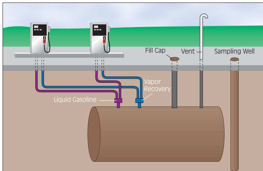
**Figure 25-69** Piping system of a gas station.
