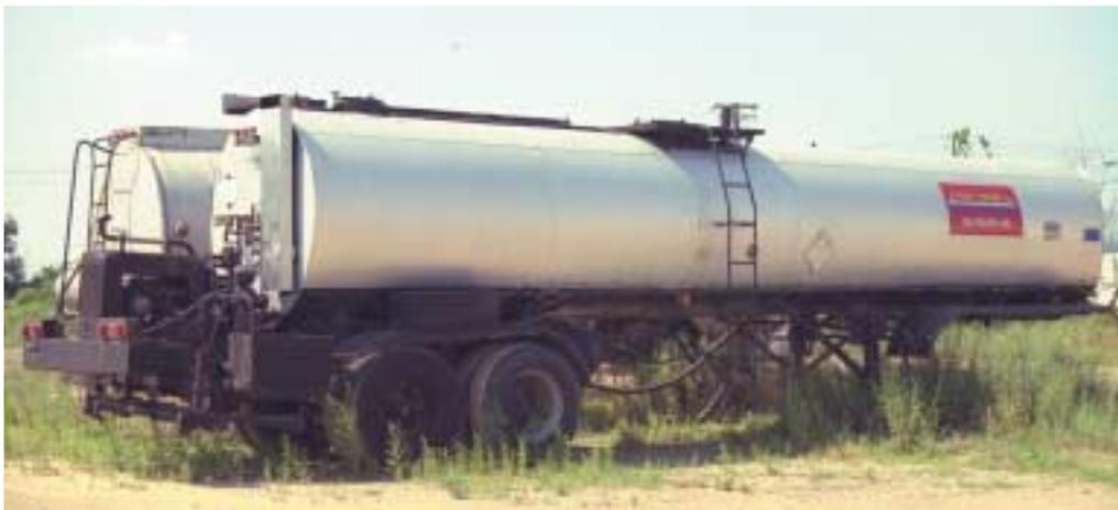
**Figure 25-59** These trucks carry molten products and can be heating the product while driving. This practice is illegal but is found on occasion. The fuels used to heat the product are either diesel/kerosene or propane.
