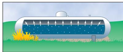
As heat increases inside of tank, the pressure also increases. The liquid will begin to boil.
