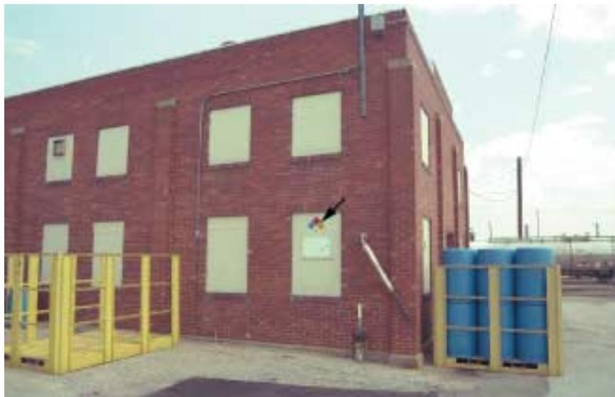
**Figure 25-4** The NFPA has developed a system for identifying potential chemical hazards in a building. The system is known as NFPA 704.
