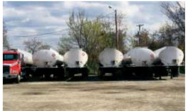
**Figure 25-42** Many of the differences between a 306 and a 406 tank truck are internal. The biggest difference is that the dome covers on a 406 are less likely to open during a rollover, although the skin of the tank is thinner. (Photo courtesy of Maryland Department of the Environment)
