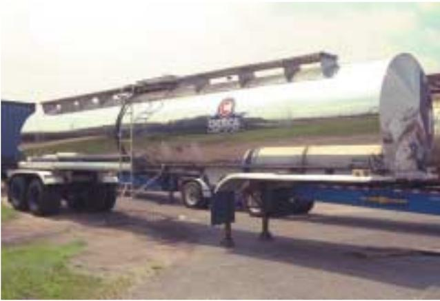
**Figure 25-49** This insulated version is identical to the uninsulated tank but has an aluminum cover and insulation. Note the differences in these two trucks. The one on the right has safety railings around the manhole. Although not an absolute rule, the truck on the right would carry more dangerous products and would have other added safety features. Most of these items are not required but were added by the trucking company.
