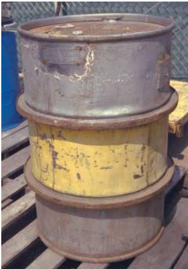
**Figure 25-32** The type of container can provide some clues as to the contents of the container. Because this drum is reinforced, it has a high likelihood of containing an extremely hazardous material.
