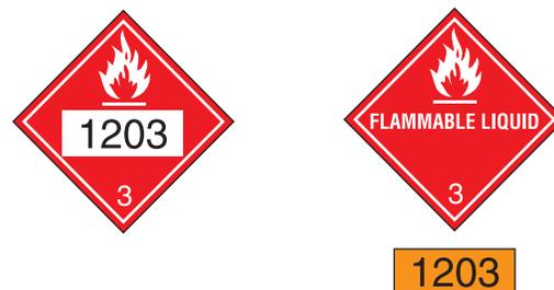
**Figure 25-7** There are three ways to signify the four-digit ID number for bulk shipments. The most common is for the four-digit DOT identification number to be placed in the middle of the placard.
