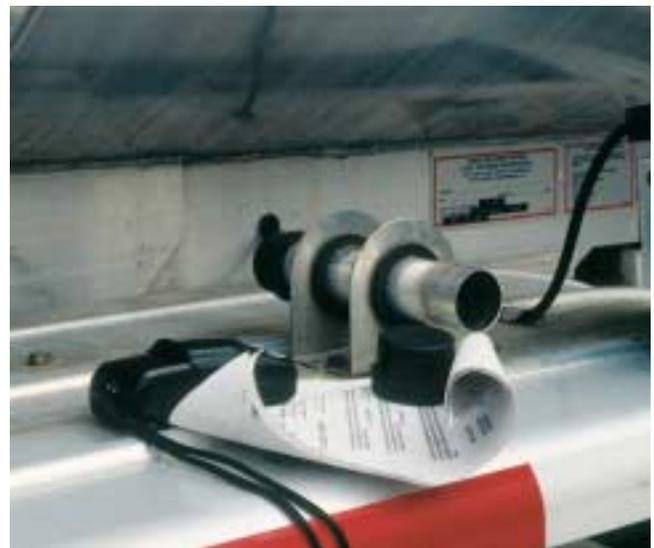
**Figure 25-43** In most cases the shipping papers will be with the driver in the cab of the truck, but they may be in a special tube located on the trailer.
