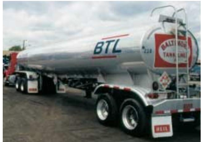
and the number of pots is indicated by the number of outlets as well as the number of manhole assemblies located on top of the tank. The maximum pressure that this truck can hold is 3 psi. The compartments are separated by bulkheads, which usually fail during a rollover situation. Although in most states the shipper is not allowed to ship a mixed load of flammable and combustible materials, widely differing loads can be encountered from compartment to compartment.
