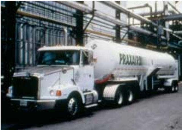
**Figure 25-55** The MC-338 carries cryogenic liquefied gases. The tank resembles a rolling Thermos bottle.
