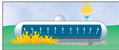
The relief valve will ignite, also causing heat to be on the tank by that flame. The pressure will increase in the tank.
