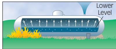
As the pressure increases, the relief valve will open, releasing propane. The propane, being heavier than air, will sink.
