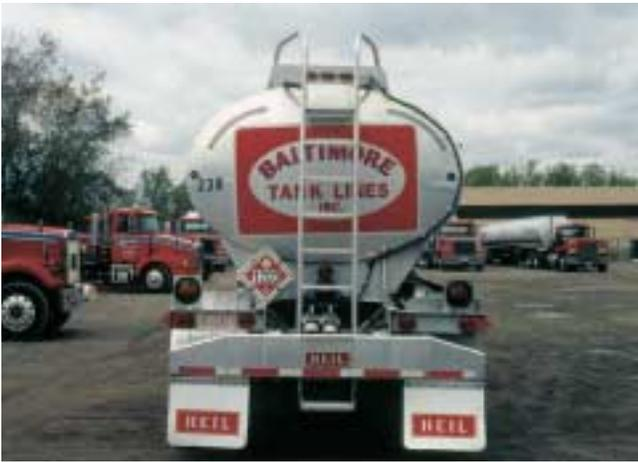
**Figure 25-44** The DOT-406/MC-306 is the most common truck on the highway today and is referred to as a gasoline tanker. It can and frequently does carry other types of flammable and combustible liquids. (Photo courtesy of Maryland Department of the Environment)
