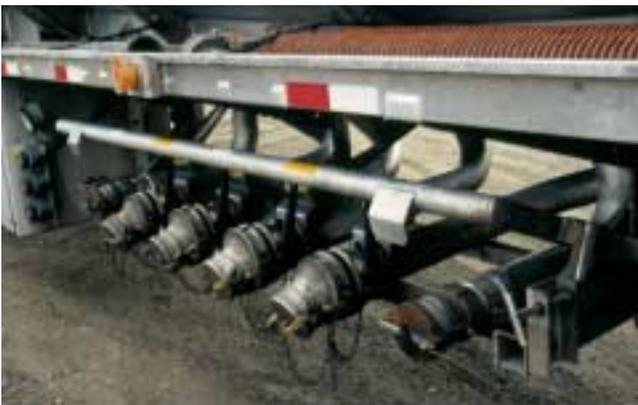
**Figure 25-45** Most 406/306 trucks have more than one tank (pots) and the number of tanks is indicated by the number of valves or the number of dome covers on top of the truck. (Photo courtesy of Maryland Department of the Environment)
