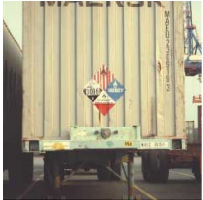
**Figure 25-5** The DOT requires some shippers of hazardous materials to provide placards to warn responders of chemicals that may be on the truck.
