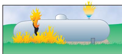
As the pressure in the tank is increasing, the tank may discolor and the pitch of the relief valve will get higher. Eventually the tank will rupture. This is known as a BLEVE.
