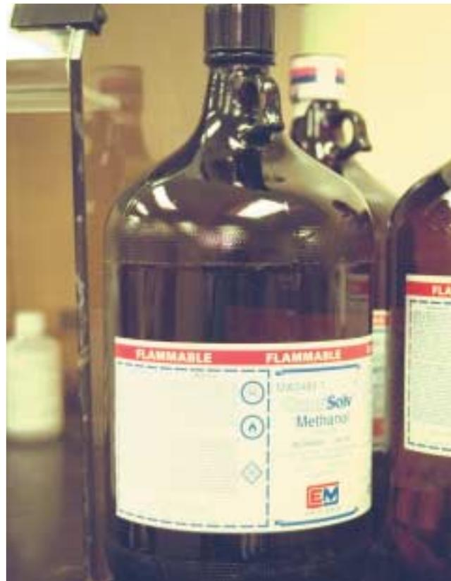
**Figure 25-35** This glass jar is coated with a plastic coating that will not allow the liquid to spill out if the glass is broken or dropped.
