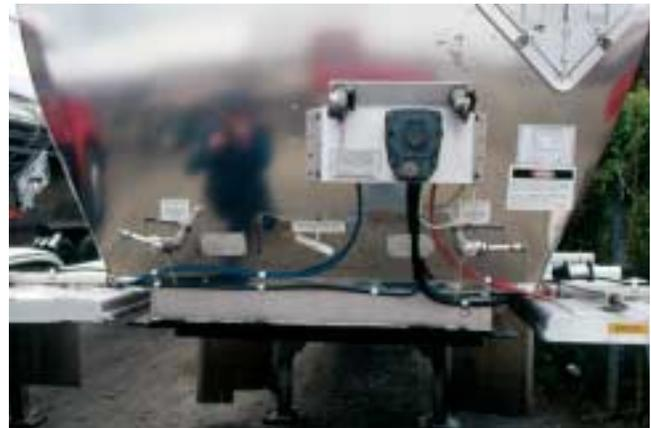
**Figure 25-50** Products carried in an insulated 407/307 need to remain either heated or cooled. Some products may need to be heated for offloading. The heater coils that run around the tank heat the product up, allowing it to be offloaded.
