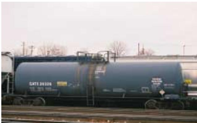
**Figure 25-65** The pressurized car is indicated by the valves being contained within the protective housing of the railcar.
