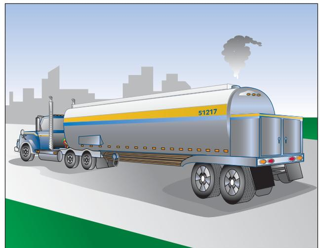
**Figure 25-56** When transporting liquids it is not uncommon to see vapors coming from the relief valves. The truck can only travel with the tank at 25 psi or less. As it heats, the pressure increases, triggering the relief valve. This is a normal situation, and the tank will vent until below the 25 psi. When offloading the pressure can be increased to assist with the offloading procedure.
