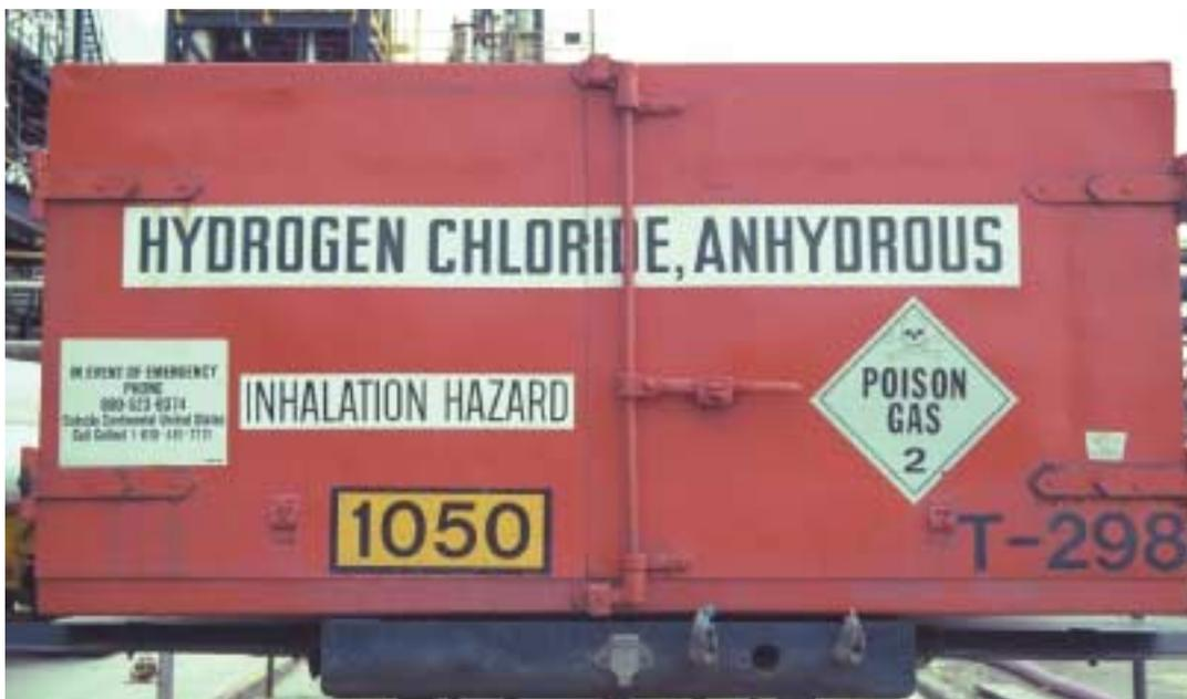
**Figure 25-24** The DOT adds the “Poison—Inhalation Hazard” label to those materials that present severe toxic hazards.
