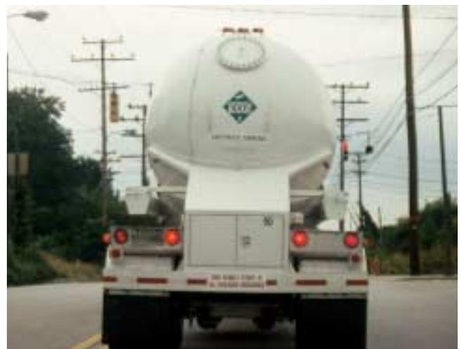
**Figure 25-53** MC-331 tanks carry liquefied compressed gases such as propane and ammonia. They are made of steel and are designed to carry a variety of products.
