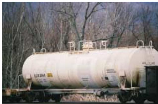
**Figure 25-66** This specialized railcar holds liquefied carbon dioxide, a cryogenic material.
