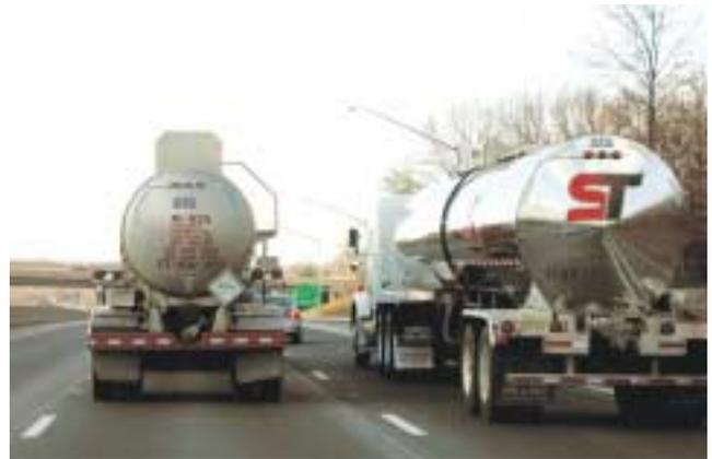
**Figure 25-48** On the right is an insulated MC-307/DOT-407, and on the left is an uninsulated MC-307/DOT-407. Both trucks hold comparable products, but the insulated one holds products that are heated or may require heating to offload.
