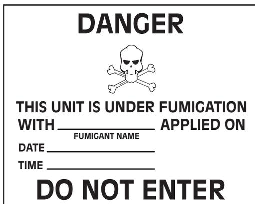
Figure 25-22 “Fumigation” marking.
