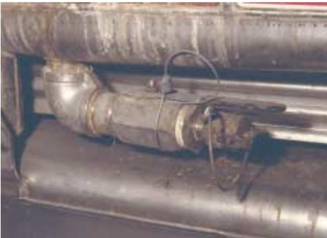
**Figure 25-40** The most common type of spill occurs when a valve is knocked off, releasing the contents.
