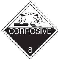
**Figure 25-6** “Corrosive” placard. Not to scale.
